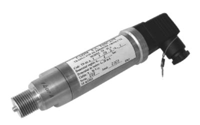
The pressure transducers type TP-01are used to make the current loop used in the industrial analogical systems for measurement, control and regulation. The transducer's connection is in two wires.
