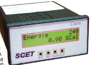
mA or voltage 0...5V. The device also has a unified signal output (4...20 mA) for recorders. For each input, a series of parameters can be programmed such as: minimum and maximum values in engineer units, the alarming values, the decimals number. The interior and exterior diaphragm diameter, the diaphragm material and the position of the pressure intake ports can be programmed.
