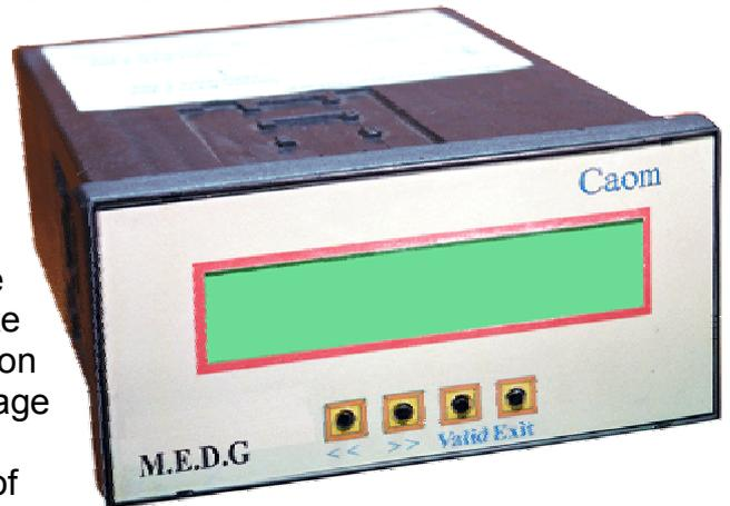
The device has a flash memory that saves the temperature, the pressure, the pressure difference and the flow counters at a programmed time interval.
